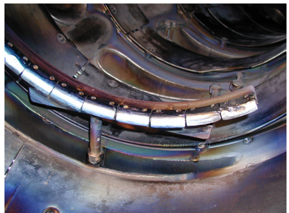
Fig. 2. Smaller and discrete molybdenum limiter employed before the year of 2000.
